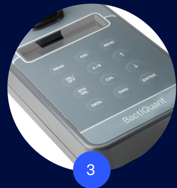
Enzyme activity is measured using a fluorometer
