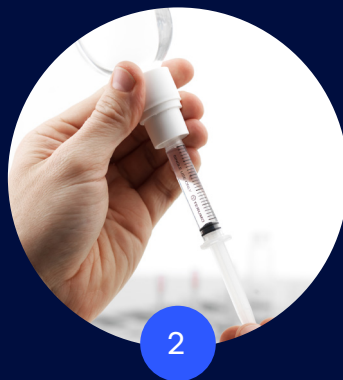
Analysis chemistry is added directly to the filter house
